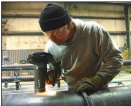
Patrick Sturgis checks a flux cored weld between passes.
