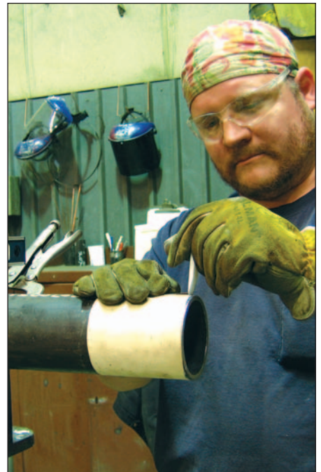
Tom Garner lays out pipe for duct burner header piping.
