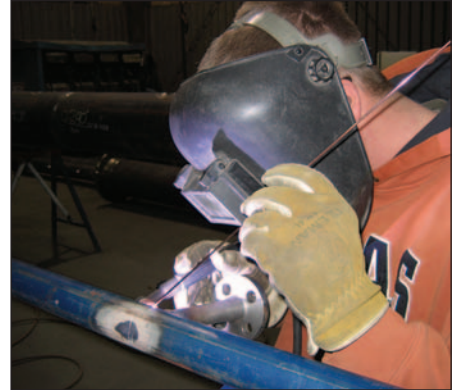
Clay Mindermann tig welds pipe for a John Zink project.
