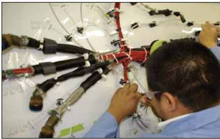
Employees at the Cherokee Nation Industries' Stilwell facility prepare wiring harnesses for a Sikorsky helicopter. The Stilwell plant has over 360 employees.
