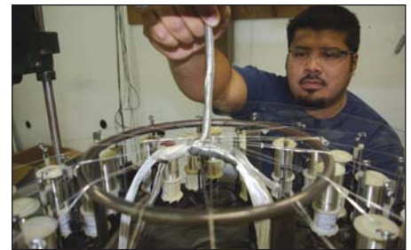
A CNI technician directs metal braid onto wire bundles for the CALCM (Conventional Air-Launched Cruise Missile) Project.
