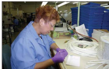
Another CNI technician marks battery cable wire for tactical quiet generator (TGQ) program.
