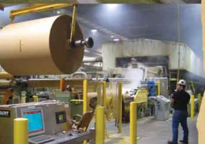
NGC employs about 80 people in the manufacturing of gypsum wallboard liner universally used in construction. Sometimes the product is described as "paper for drywall."
